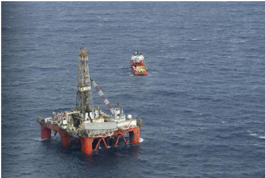
Figure 3: *Ocean Patriot* semi submersible drilling rig
